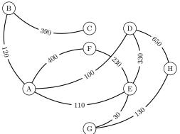
Apply Dijkstra's algorithm to find a minimal path from the vertex H to the vertex B. Illustrate the sequence of graphs  $T_0, T_1, \ldots$  which arise during the process.
